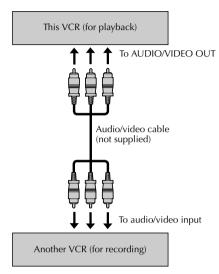
When using this VCR as the recording VCR, connect this VCR's audio/video input connectors to the audio/video output connectors on the other VCR. If the playback VCR is monaural, connect the audio output connector on the playback VCR to the left audio input connector on this VCR.
